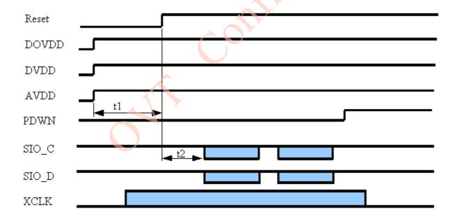
t1: from powers on to SCCB software reset, >= 3ms
