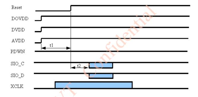
t1: from powers on to SCCB software reset, >= 3ms
