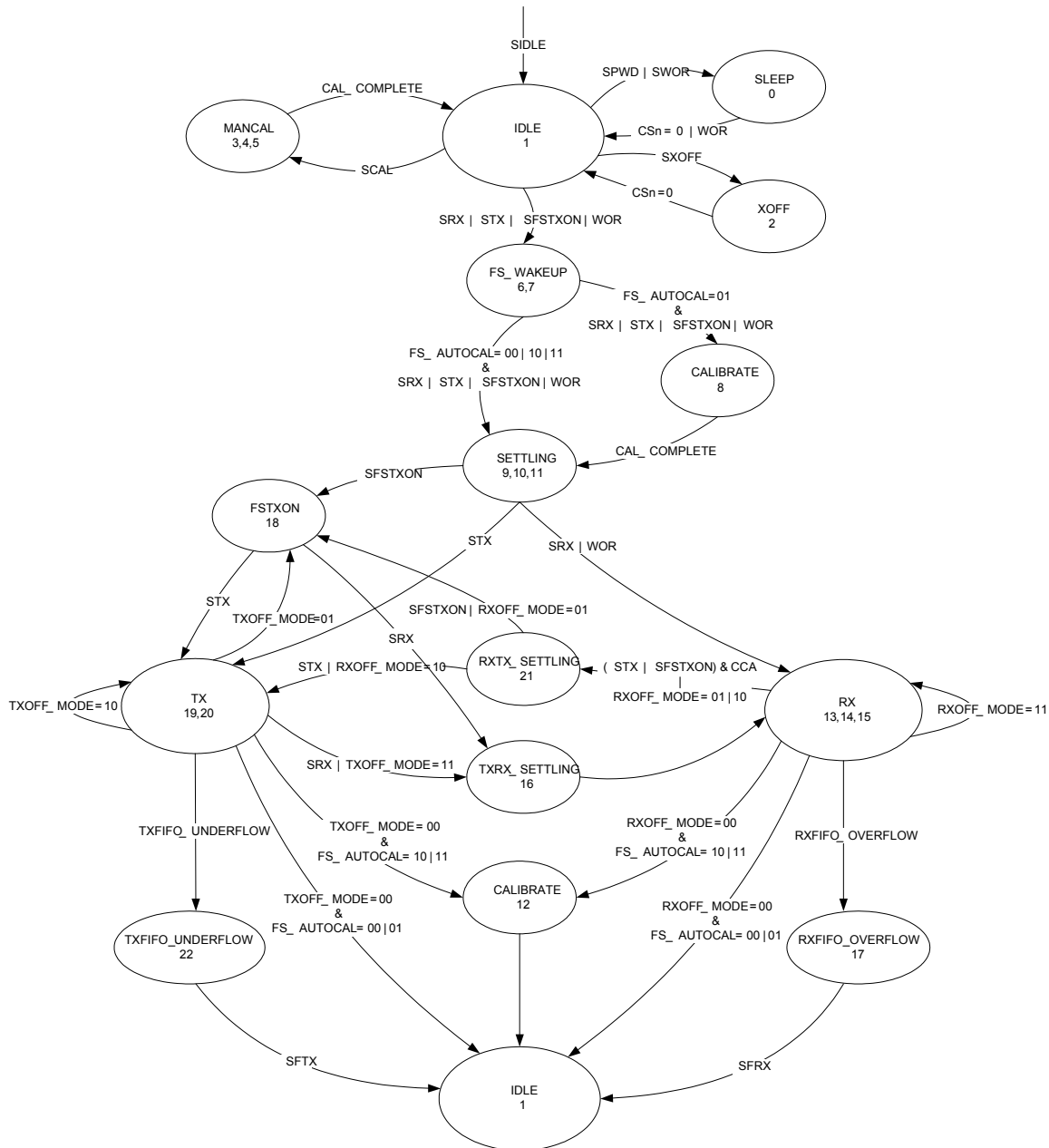
Figure 15: Complete Radio Control State Diagram
