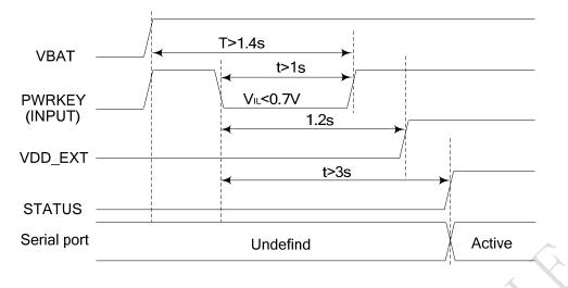
Figure 12: Timing of power on module
