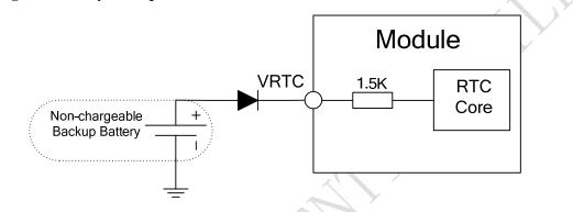
Figure 16: RTC supply from non-chargeable battery
