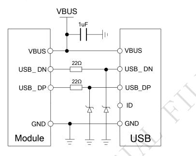
Figure 23: USB reference circuit
