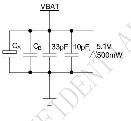
Figure 5: Reference circuit of the VBAT input
