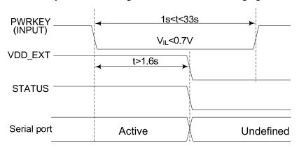
Figure 13: Timing of power down SIM800C by PWRKEY
