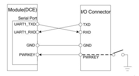
Figure 24: Connection for software upgrading and debugging
