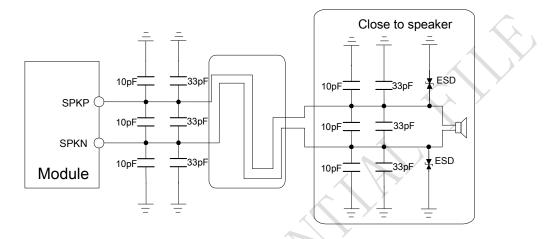
Figure 29: Speaker reference circuit
