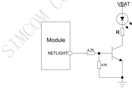
Figure 35: Reference circuit of NETLIGHT
