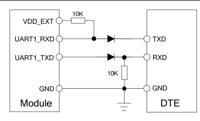
Figure 20 : Diode isolation circuit
