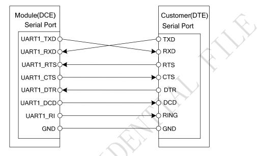
The following figure shows the connection between module and client (DTE).
