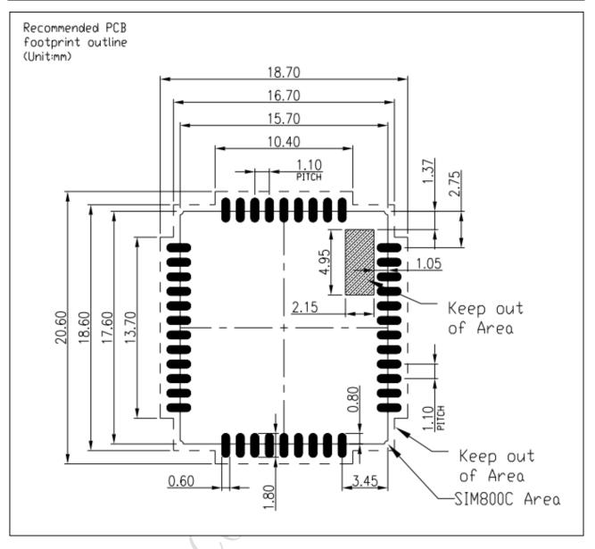
Figure 4: Recommended PCB footprint outline (Unit: mm)
