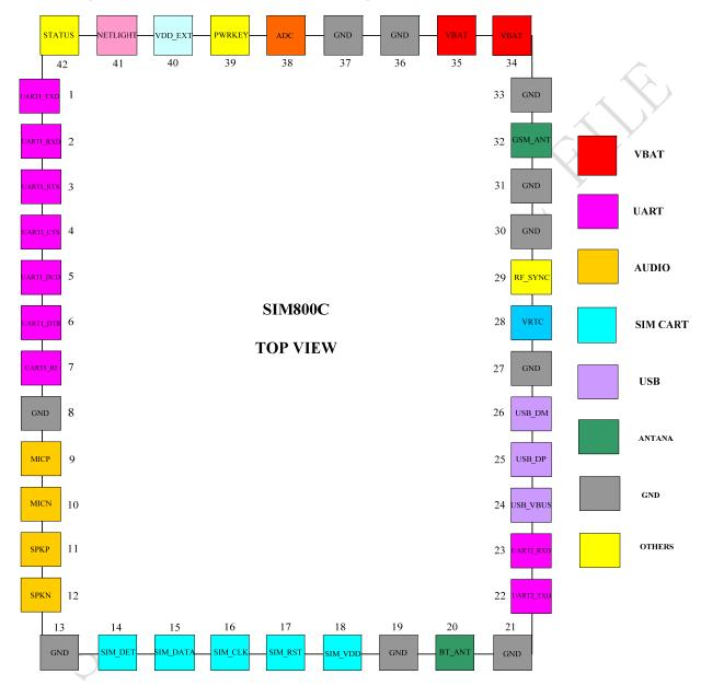
**Figure 40: Pin assignment**
