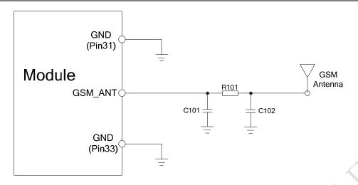
Figure 38: GSM antenna matching circuit without RF connector
