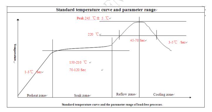
Figure 42: Typical solder reflow profile of lead-free processes
