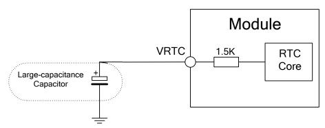
Figure 15: RTC supply from capacitor
