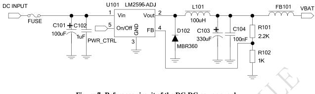
Figure 7: Reference circuit of the DC-DC power supply
